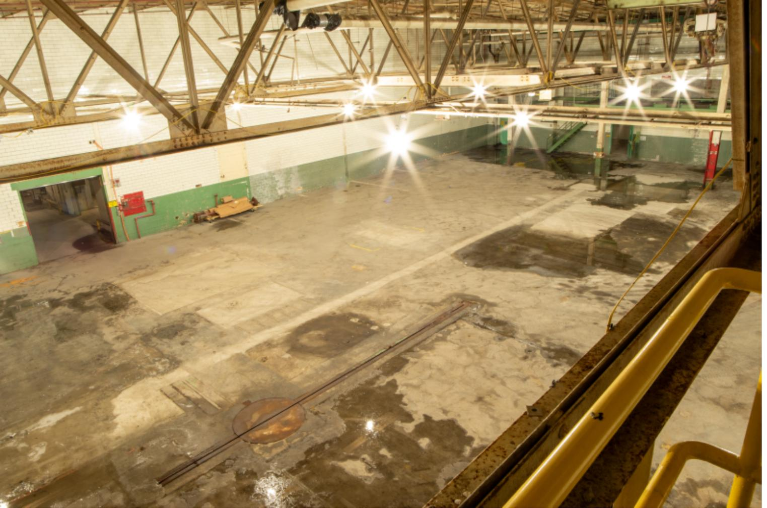
*Both photos are of the finishing room. The floor used to flip down and paper would move by elevator down into the new trainshed or warehouse to be loaded onto rail cars, trucks or stored. Both photos December 31, 2024, Joey Kelley, JoeyKelleyPhoto.com*
