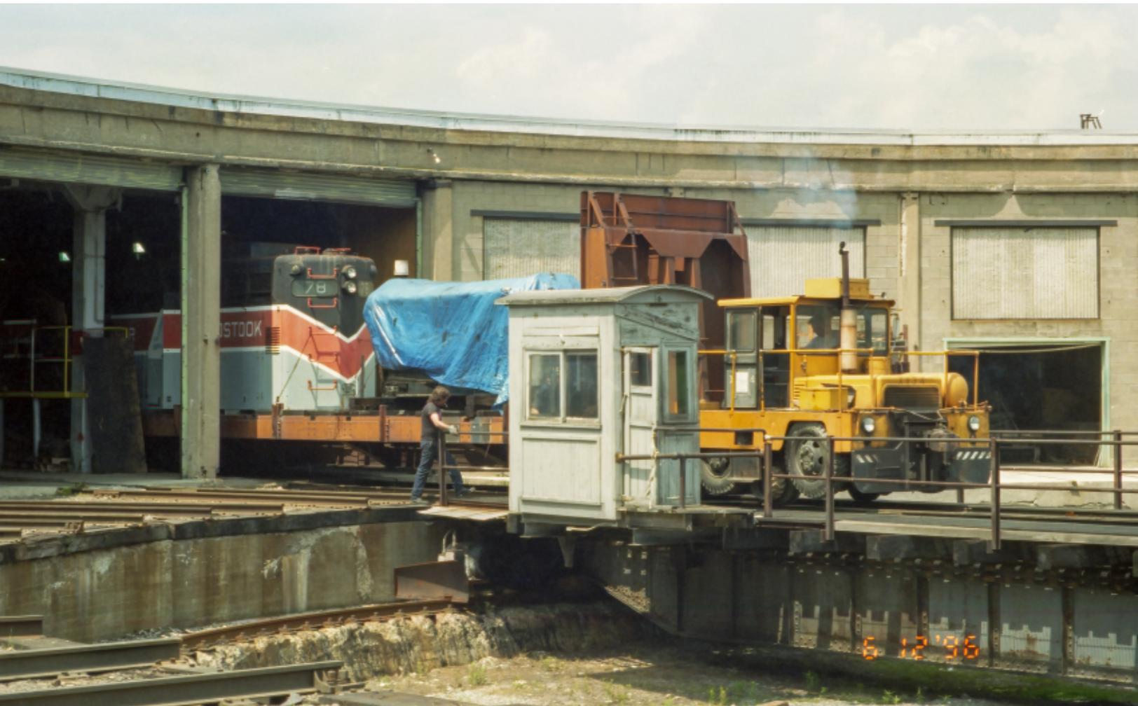
*Perhaps the least photographed of all the types of equipment on the B&A, trackmobile X-134 is being used to pull on the hood and prime mover of 78 while both are on a former pulpwood flat. Northern Maine Junction, June 12, 1996, Mike Guay photo, JoeyKelleyPhoto.com Collection*
