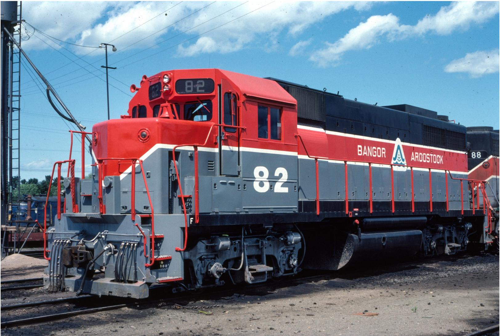
*Above: David Hamley photographed 82 at NMJ on June 10, 1981 – she was painted in May of 81 into this scheme. Note the Nose bell that has been retained. 82 also has a winterization hatch over its front cooling fan (box looking affair over the forward of the two cooling fans on the rear of the long engine hood) this was the only GP38 to have this hatch.*
