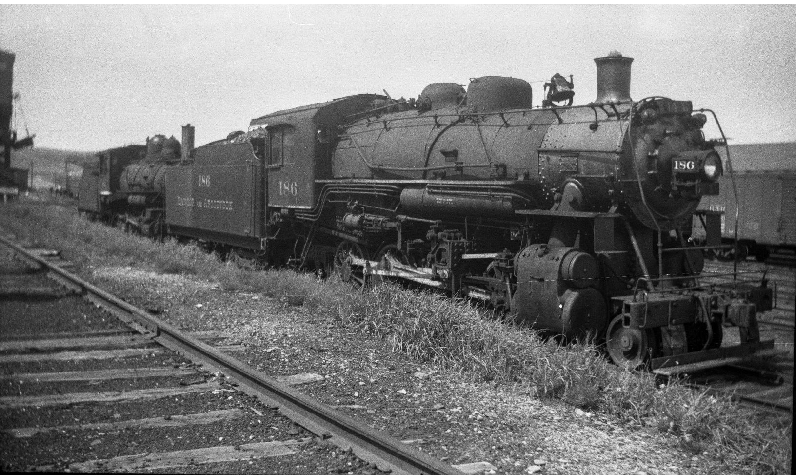
Photographer W.H. Allen shot 186 at Van Buren in August of 1949. Note that both the locomotives have their stacks capped. (rocks are holding the caps down) Diesels were very much in place by 1949. JoeyKelleyPhoto.com Collection
