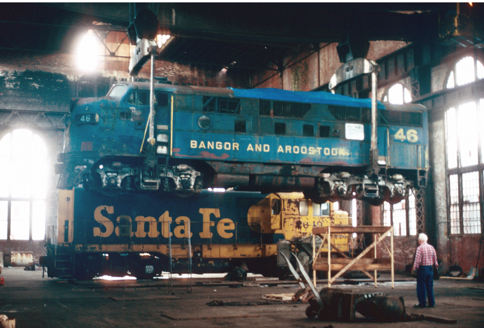
46 proves that locomotives were not meant to fly, but fly they must! This 1988 photo inside the Reading, PA shops shows 46 and the donor CF7 used for parts. Richard Jahn photo
