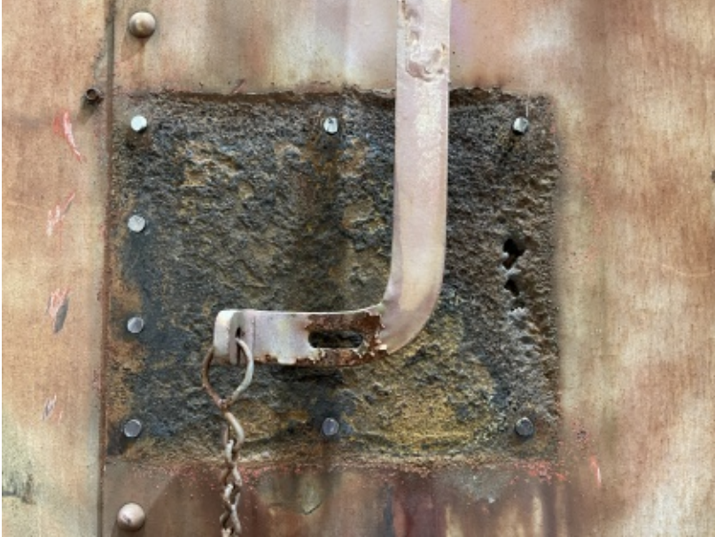
Above: The original Ventilator controls were unable to be salvaged. Right: The new ventilator controls, reproduced from the originals, look right at home on the restored car. Both photos Howard Pincus
