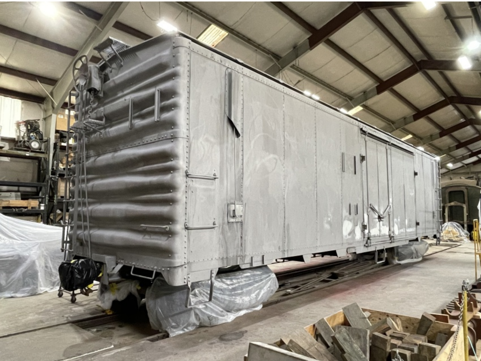
Above: Blasted but before primer, 2569 looks like an undecorated model kit, but in 1:1 scale! July 23, 2024, Howard Pincus photo
