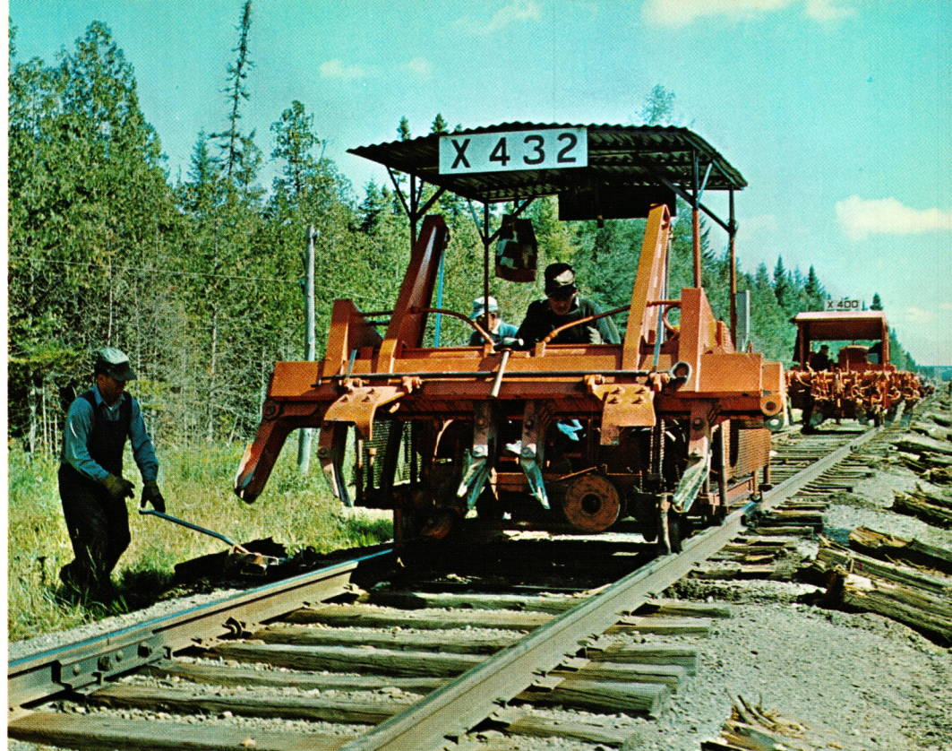
Getting Ready for a New Tie —This track scarifier works in conjunction with the machine shown on the page opposite. It prepares the way for the insertion of a new tie.
