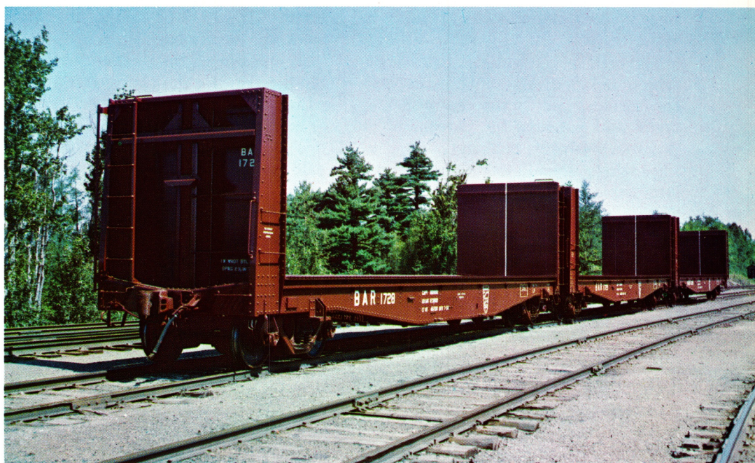
They Come Even Larger These Days —These end rack pulpwood cars, with a 22-cord capacity, were the last word in this type of equipment when they were acquired by the Bangor and Aroostook in 1954. Today, however, they are dwarfed by 168 cars purchased in 1964 that are 64 feet long and can carry 32 cords.
