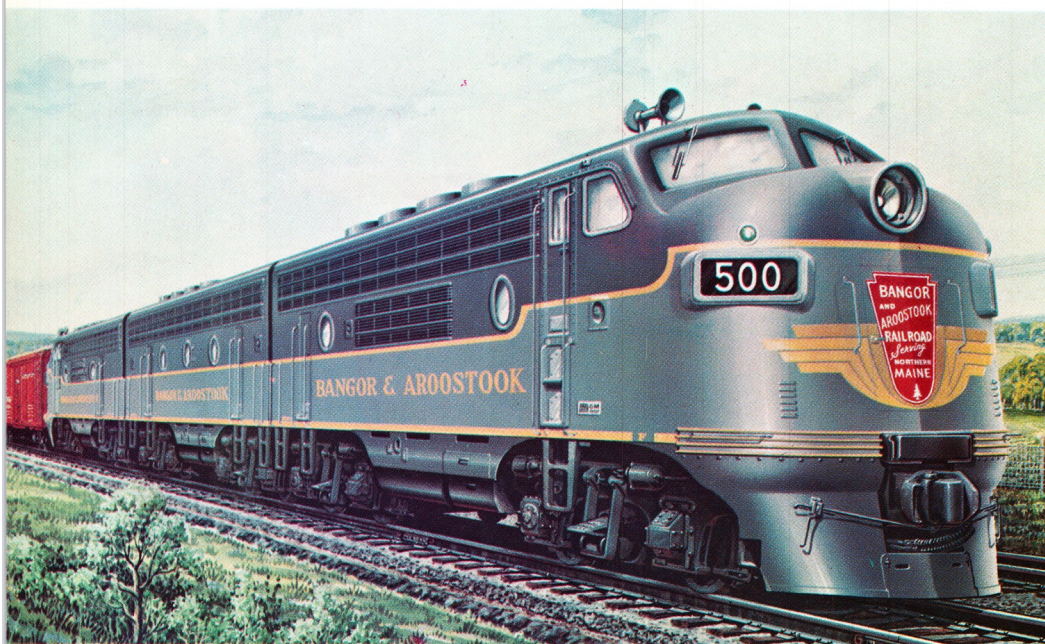
The first break with steam power— This “A” unit and its two accompanying “B” power units were the first diesel locomotives purchased by the Bangor and Aroostook. The supplier was the Electro-Motive Division of General Motors. All of the “B” units have since been replaced by units that are independently operable.
