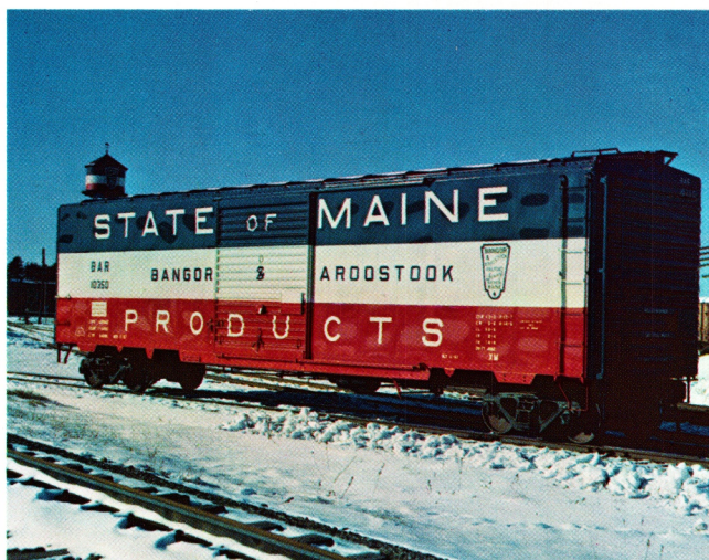
For paper tonnage —This is one of the Bangor and Aroostook's 50-foot box cars equipped with a cushion underframe. These cars, of which another 400 were ordered in 1965, were acquired for paper traffic.
