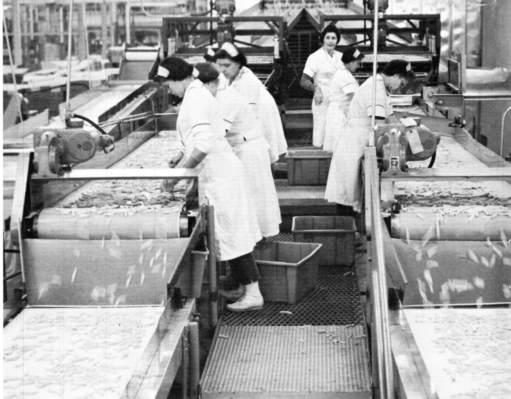
One Step in a Quality Control Program —Workers in an Aroostook frozen foods plant inspect sliced potatoes for discolor or any other blemish that makes them substandard as one of the several quality control inspections that are inherent in the production of french fried potatoes.
