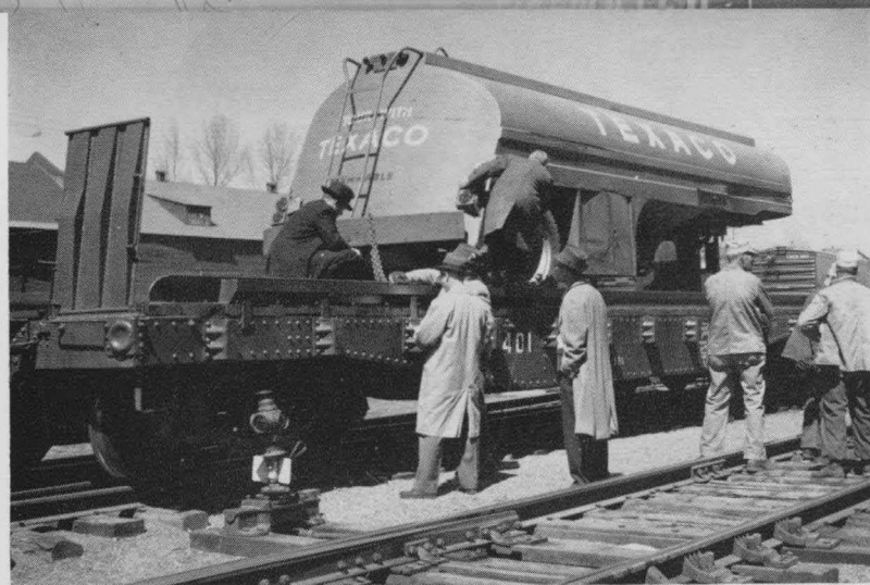
Above, impact tests are made with a tank trailer on a piggyback car to determine if tanks can be used in piggyback service. Preliminary tests were successful, observers said. Below, 13 cars of steel for the construction of a Snark launching site await unloading at Presque Isle. 65 of the 70 cars of steel for the site have already arrived.
