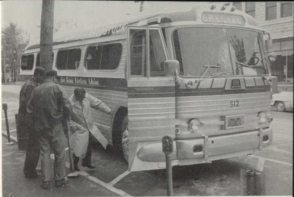
General Motors District Manager Henry Hickman, pointing, explains principle of "air bellows" suspension system to interested bystanders. The new system replaces conventional metal, leaf springs.
