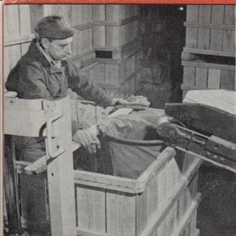
Heavy canvas chute is used to prevent potatoes from bruising as they drop into pallet box. Similar chute is used in East Hartford when boxes are emptied.
