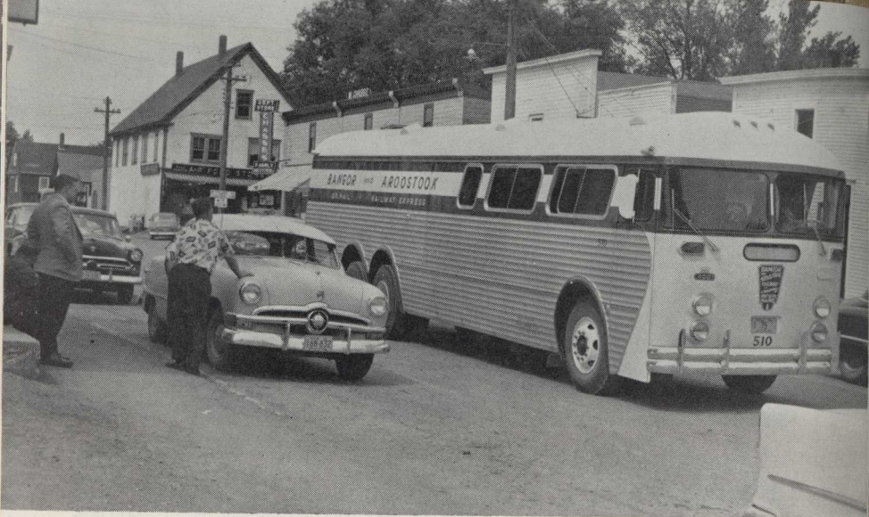
New Bangor and Aroostook bus, a Crown super cargo coach, attracts curious glances as it stops in Ashland on inspection tour June 20. The bus is a new type carrying 20 passengers and has a cargo section 20 feet long. It was developed on the West Coast during the last two years and was purchased, according to Highway Manager Arnold J. Travis, as a vehicle well-suited to the Ashland Branch run.
