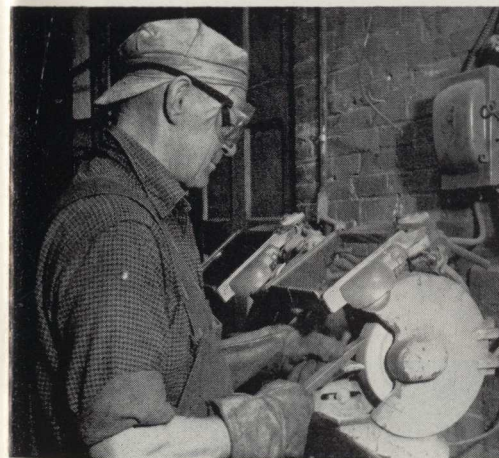
At left, Carpenter O. S. Heal, Derby, shows the proper use of protective devices for grinding with an emery wheel. The tool rest should be within one-quarter of an inch of the wheel and under no circumstances should tools be ground on sides of wheel. In addition, all protective devices provided for the wheel itself should be in place, and the operator should use safety glasses and coverall goggles.
