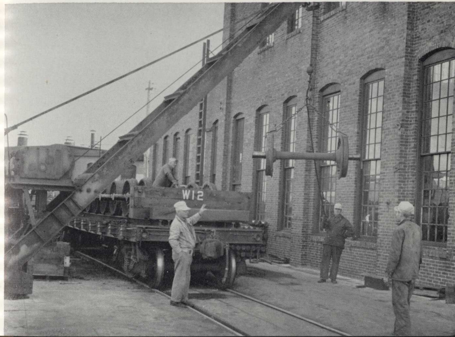
Below, Laborer W. T. Bohan, Yard Foreman M. A. Furlong, Burro Crane Attendant J. J. Willinski, and Burro Crane Operator R. E. Jay demonstrate proper safety practice while loading heavy equipment with crane. Note that each man is safely out of the way if the load should break loose.
