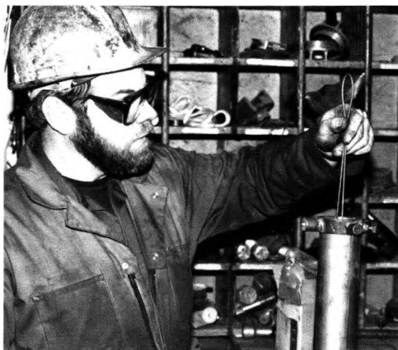
Hoists and jigs make it possible for one worker to do a job that once required at least two and sometimes more. At left, Lavin inserts a rivet into a brake cylinder tube prior to fastening the assembly by pressing it over a mandrel. Lavin devised a way to use seamless tubing available over the counter instead of buying the entire assembly at a cost of $128 each, a savings of nearly $100. Below, Lavin uses a Porta-power tool and a jig of his own design to press a bushing into the truck assembly. The previous procedure was for one man to hold the part while his partner hammered it in. Lavin thinks his way is safer and faster.
