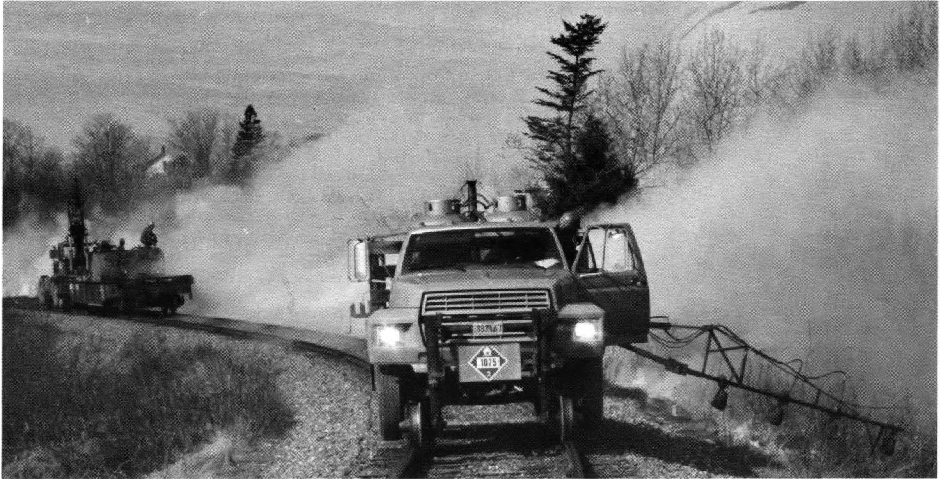
The right-of-way burner operated by Bryce Clark, who did much of the fabrication work on the project, was the product of a TQ Action team including Clark, Brent Brewer, Bob Cote, Aaron Picken, Fred Rolfe, and Jerry Toner. State law requires the railroad to burn its right-of-way in the spring. It has been a labor intensive process and the propane-fired burner has made it much more efficient.
