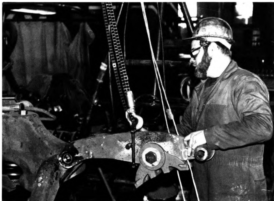
Hoists and jigs make it possible for one worker to do a job that once required at least two and sometimes more. At left, Lavin inserts a rivet into a brake cylinder tube prior to fastening the assembly by pressing it over a mandrel. Lavin devised a way to use seamless tubing available over the counter instead of buying the entire assembly at a cost of $128 each, a savings of nearly $100. Below, Lavin uses a Porta-power tool and a jig of his own design to press a bushing into the truck assembly. The previous procedure was for one man to hold the part while his partner hammered it in. Lavin thinks his way is safer and faster.
