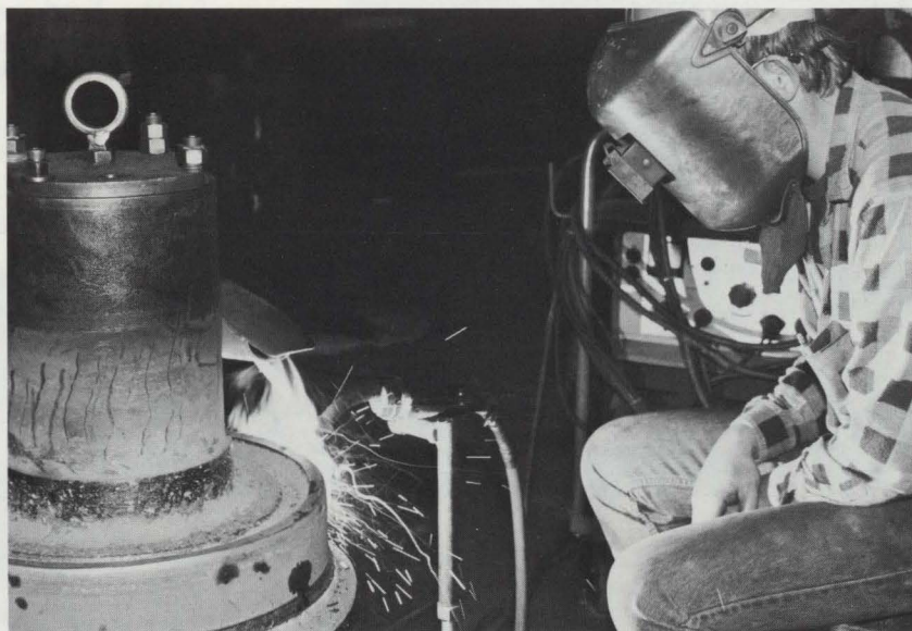
Carey's ingenuity reduced the hours to complete a wheel to 8-3/4, cutting $700 a wheel in labor costs. Now he checks his work every eight minutes instead of constantly bending over the frame and building up the wheel by hand with the stick welding process.
