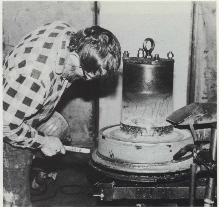
Carey removes slag from the welding process. Before he built his machine, the welding was done by hand. The challenge, he says, was to calculate the correct speed the wheel turns in order to automate the process.
