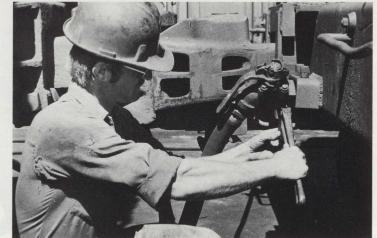
Car Repairer Paul Shields, Jr. demonstrates the repair he was making on an air hose coupling using a torch when it ignited. The gasket inside the coupling exploded driving dirt and rust particles into Shields' face. His safety glasses prevented a serious injury.
