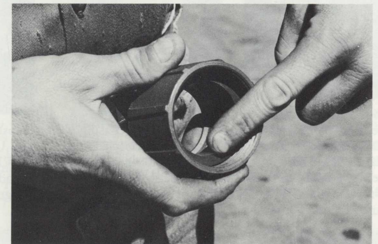
This is the gasket inside the coupling which became volatile and exploded under the heat of Shields' torch. As a result of the accident, workers are required to wear face shields as well as safety glasses. The accident was the first recorded instance of a gasket exploding under heat.
