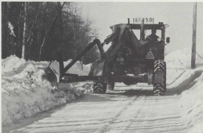
Using the new rig an operator using a Pettibone can keep roadways as well as tracks clear of snow. Toner plows several miles of roadway for the railroad in the Northern Maine Junction area.
