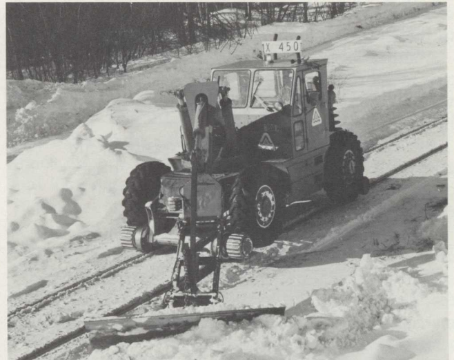
The Toner design features an 8-foot plow with live hydraulics that can be used to clear the edges of track to provide walking space for trainmen working in yards.
