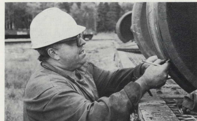
Before the new wheels are installed, Sholler gauges and inspects them.
