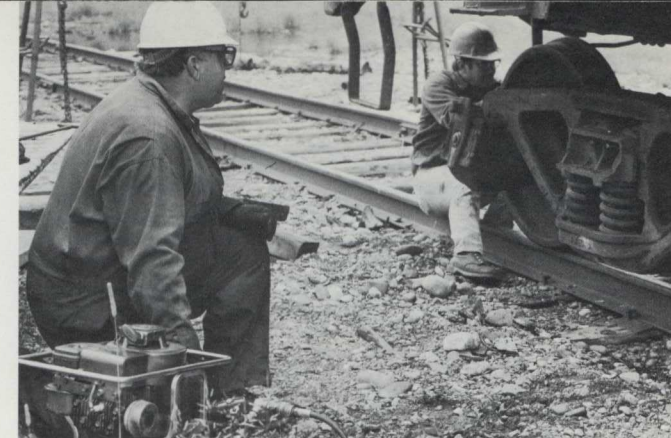
Sholler and Kevin O'Connor, who has the same kind of job in the Presque Isle area, use a hydraulic jack to change out a set of wheels on a car that's been crippled at Moody Siding.
