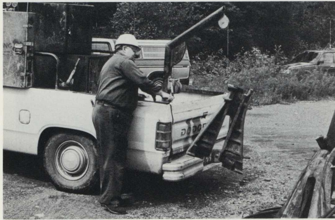
Jim Sholler's truck is a legend among the train crews and others he works with. The crane arrangement is his own design and fabrication project. Here he uses it to lift a 170-pound locomotive grab into the bed of his pickup truck.
