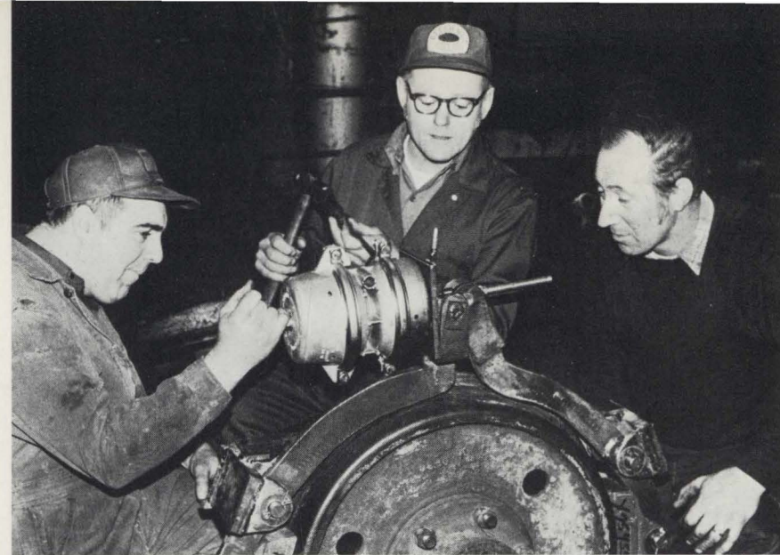
As a result of safety suggestions, workers at the Houlton Shops have designed a fail-safe brake system for self-propelled maintenance machines. The factory design lacked a backup system which has been incorporated into the new design at a significant cost saving. Pictured are Mechanics Kerry Bartlett, David Grant and Richard Simpson.
