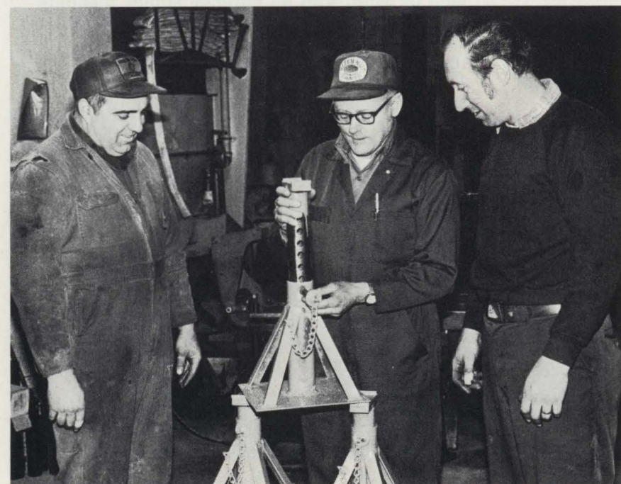
Kerry Bartlett, Dave Grant and Richard Simpson of the Engineering Department's maintenance shops designed and built the equipment support pictured here for use by mechanics who repair heavy roadway equipment in the field. The equipment was formerly supported by wooden blocking which was inconvenient and unstable. The suggestion came out of a safety meeting.
