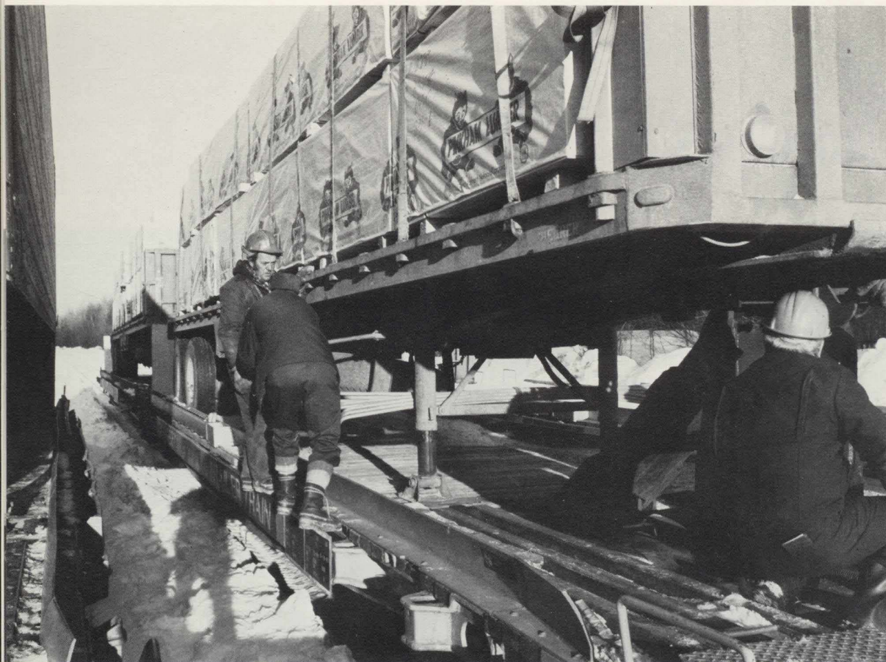
Bangor and Aroostook employees from the car repair tracks prepare a trailer load of Aroostook County lumber for unloading at Northern Maine Junction. At the lumber mill site, the cars are not deramped but are loaded while actually on the piggyback flats, making for a faster turnaround time. Price is lower than truck transportation and service almost comparable.
