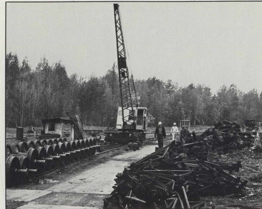
Above, crane equipped with a powerful magnet is used at Derby Shops to pile scrap for loading. Below, right, special train at Oakfield moves scrap materials collected on the Northern Division to Derby. Operation Cleansweep generated some 1300 tons of scrap and surplus material. The scrap value is estimated at $60,000 and usable materials at $23,000. The major benefit of cleansweep is a clean and safer workplace.
