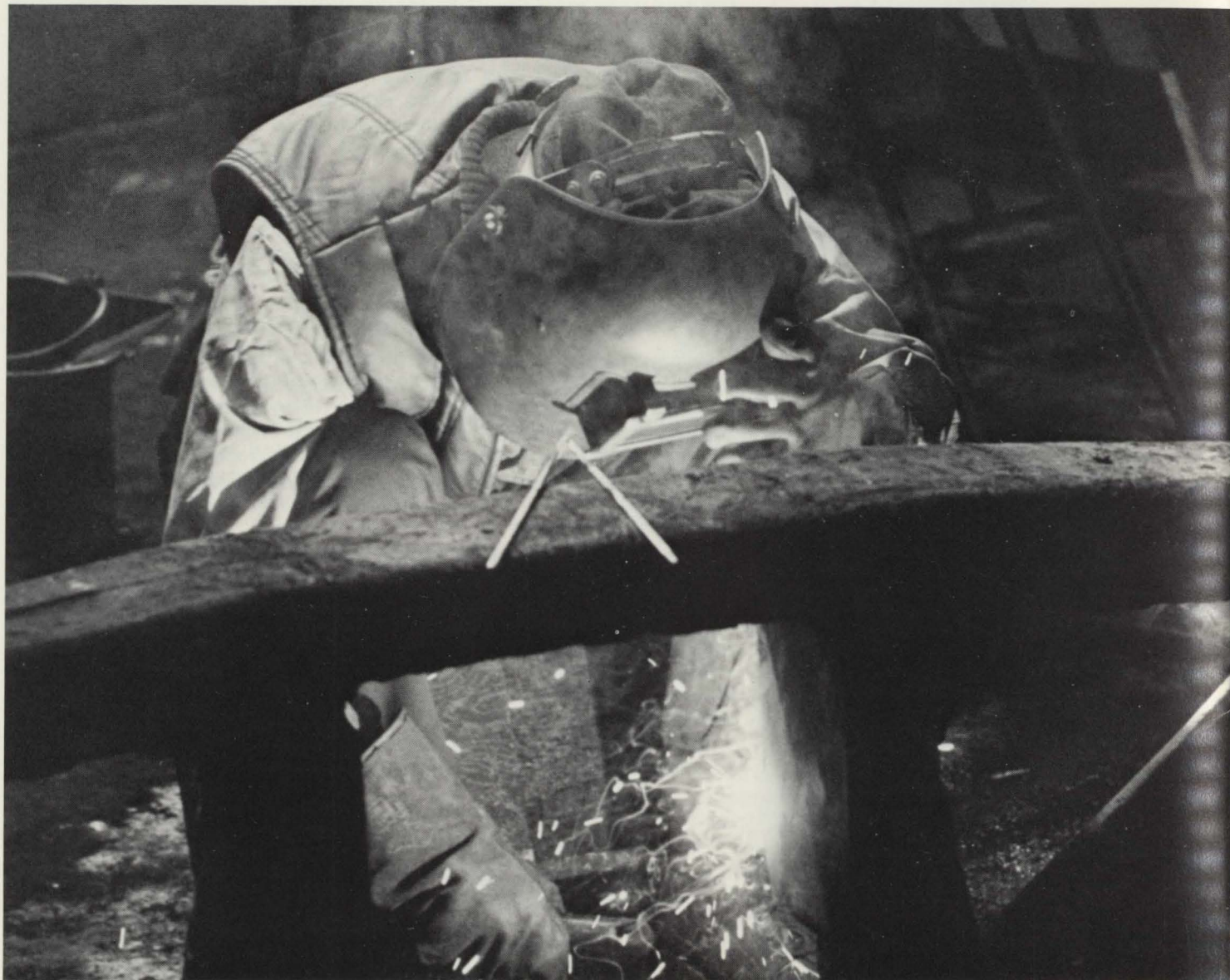
A car repairer at Derby Shops welds wear plates on a boxcar truck frame for a boxcar being rebuilt at the facility. Employment at Derby is at a seven-year high as a result of extensive car conversion programs to provide cars for International Paper Company's expanded mill at Jay.
