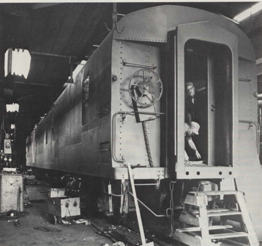
Crews at Derby Shops work on one of three 80-foot CP Rail baggage cars that will be used by the BAR as outfit cars. The baggage and express cars were built during the 40s and 50s and cost an estimated $50,000 to convert.
