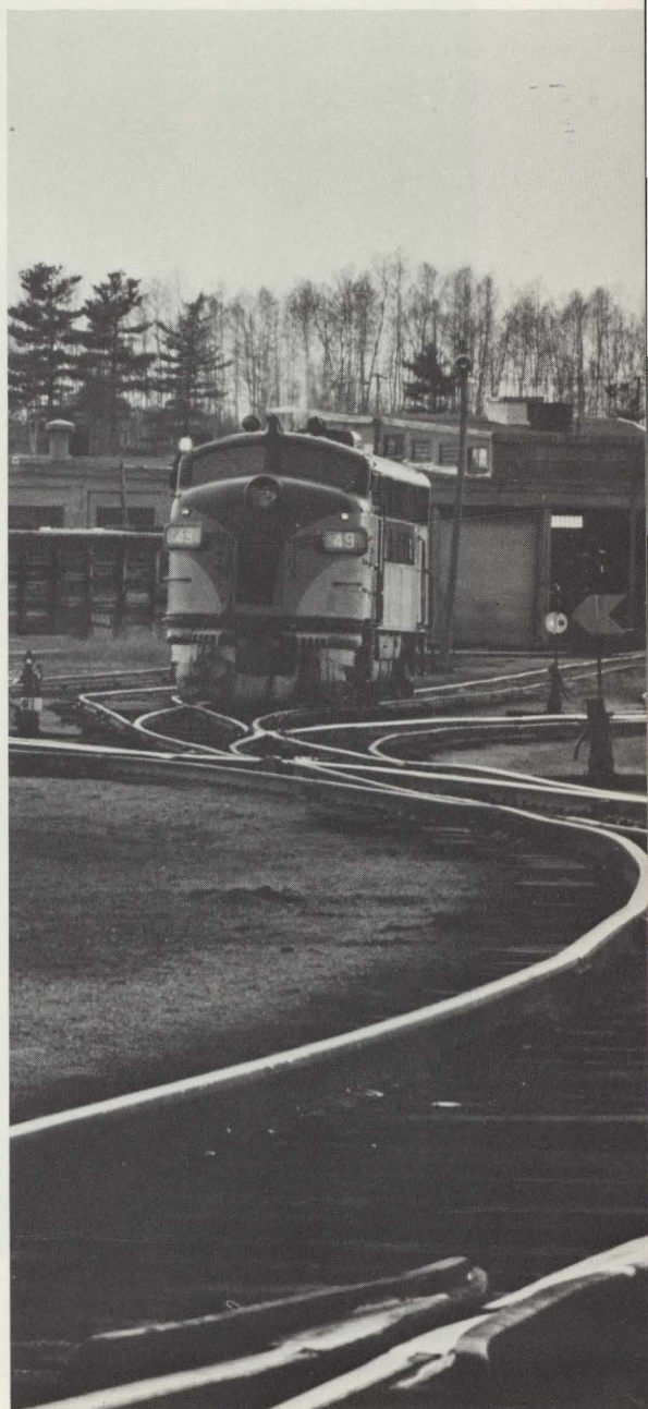
Unit 49, pictured at twilight at the Northern Maine Junction diesel shop, is one of three units equipped by the DOT with experimental strobe units. One lamp of the flashing unit can be seen at left of the cab at top.
