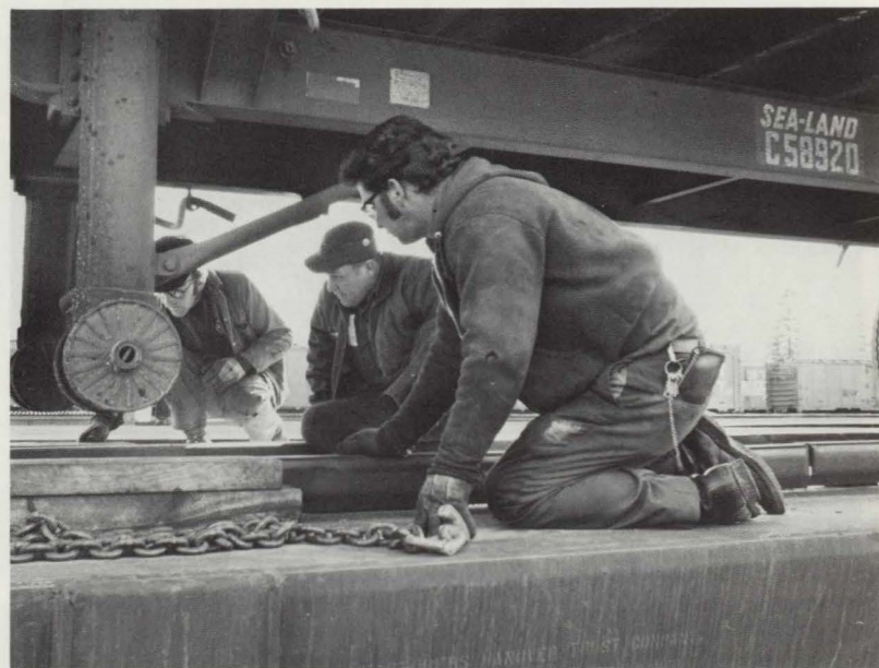
Car Repairers John P. Withee, left, and Leland Nowell, right tie down a Sea-Land trailer at Northern Maine Junction as Fox & Ginn Driver Carl Hammond watches.
