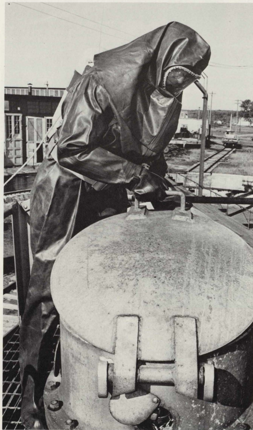
Welder Galen Carey, Derby, who doubles as a member of the railroad's wreck crew, simulates emergency conditions on a tank car containing hazardous materials. The special suit, gloves and the air pack are part of the railroad's array of protective clothing and devices employees use to perform hazardous tasks. Protective devices range from simple elastic leg bands to secure pant legs to sophisticated coverall devices with breathing apparatus.
