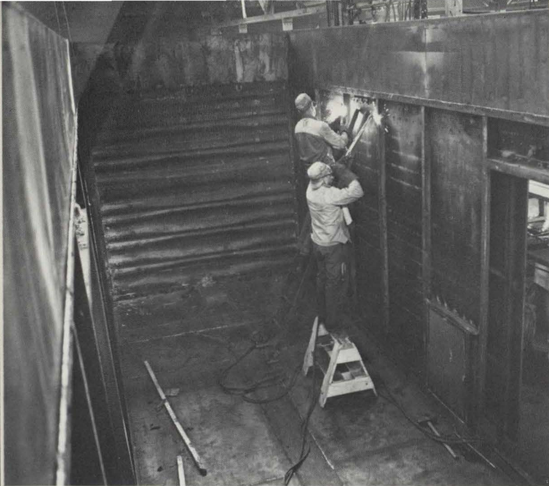
Frank Hamlin and Earl Rhodes (left) use torches to burn off adhesive left from the removal of insulation from the car. Middle, John Ellison and Tom McLean use a hoist to remove side frame to repair trucks. Lower picture, Bernard Ricker and Charles Clark use a jig to fabricate the side extension for the car. Below, Everett Black welds bracket on the chip car.
