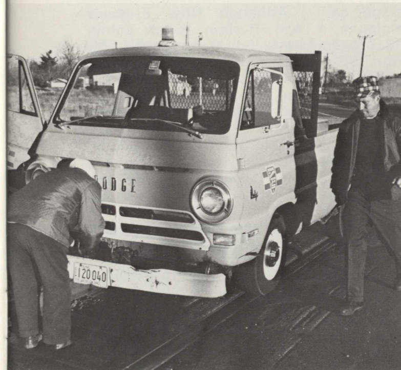
The method of track inspection was changed during 1971 so that four full-time inspectors equipped with hy-rail trucks, as shown above, now perform all track inspection.
