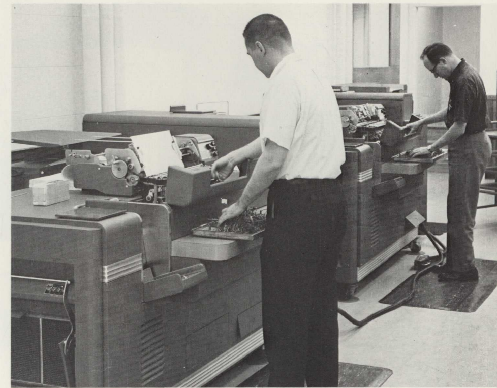
The railroad's unit record data processing machines, pictured above, are obsolete. Class I railroads are 95% computerized and the non-computerized railroad is under a severe handicap. The BAR's system is expected to be operational in May.
