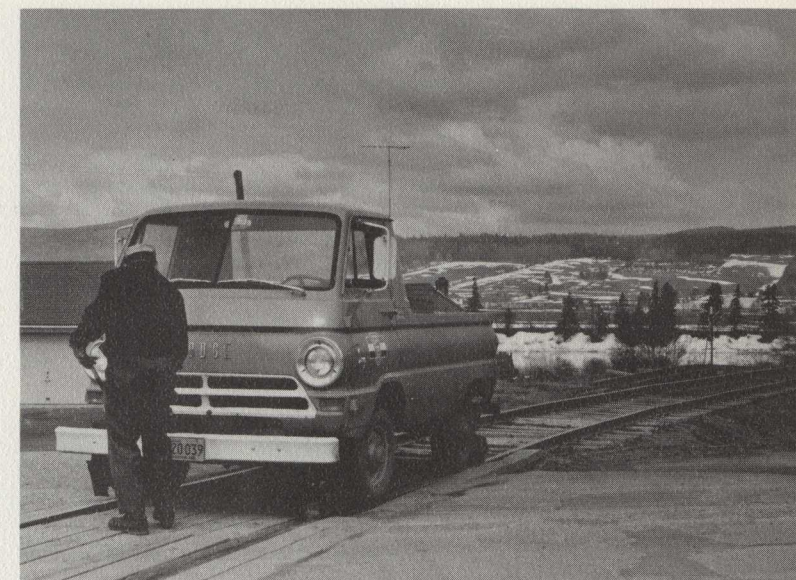
Charlie Wilson finds both the cab and the visibility from it, left photos, a great improvement over inspection from a motor car. The vehicle is easily put on the track at crossings, above, and removed. Cab is protection against the elements and the vehicle's two-way radio makes coordination with train movements safer and easier than inspection with a motor car.
