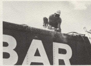
Left, Purchases and Stores workers tip the underframe off the trucks of a dismantled car. Above, a worker using an acetylene torch begins cutting up a 5000 Series box car.
