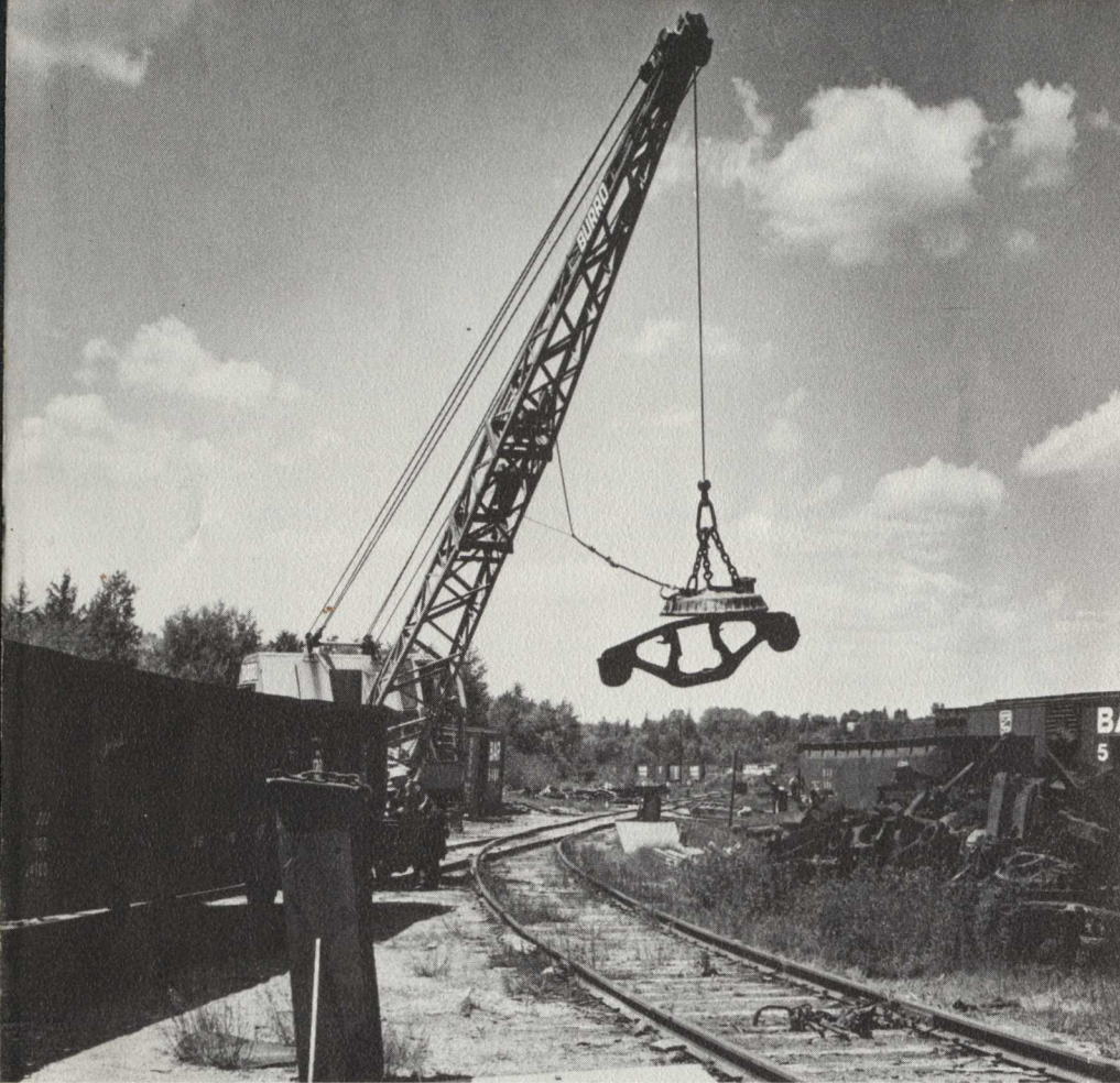
Workers use a Burro crane equipped with an electro magnet to load a truck side frame from a scrapped car at Derby Shops.
