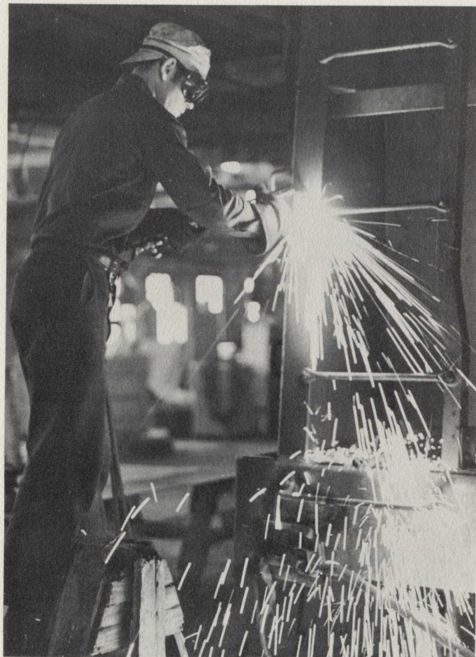
A ladder is repaired as part of the conversion program by the railroad of 72 end rack cars to lumber cars for the growing traffic in that industry.
