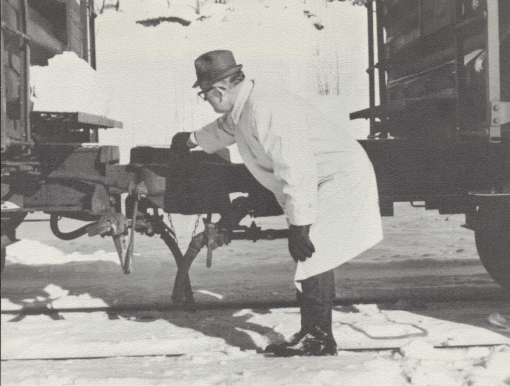
The amount of movement possible in cars equipped with a cushion underframe device is illustrated in these photographs showing the device compressed, above, and extended, below.
