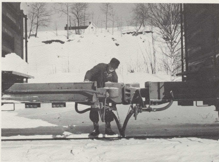
The amount of movement possible in cars equipped with a cushion underframe device is illustrated in these photographs showing the device compressed, above, and extended, below.
