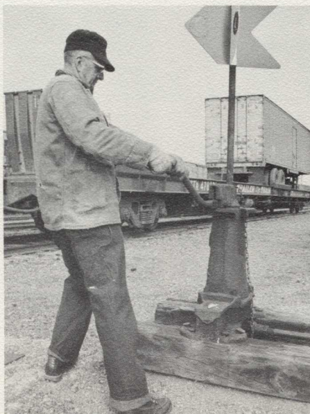
The body must be in the proper position in throwing a switch or the brakemen can lose footing if the handle sticks, then lets go.
