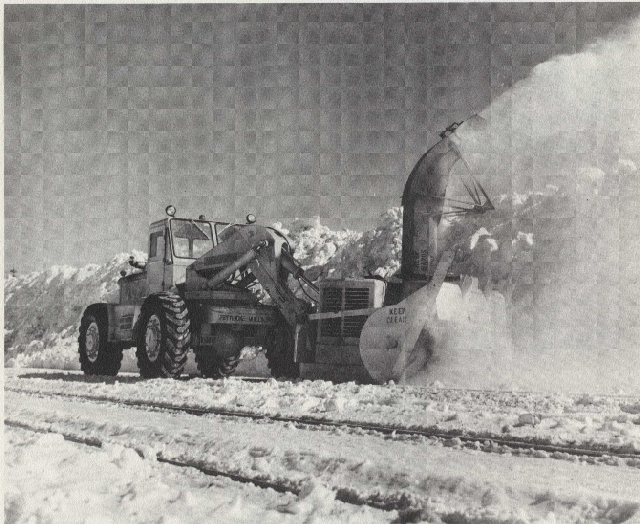
A large snowblower attached to a Pettibone Milliken cleans snow from the edges of Oakfield yard after the spreader has 'swept' the snow to the edges. Machines like this have taken much of the physical backache (and some of the headaches) from the railroad's snow removal chore.
