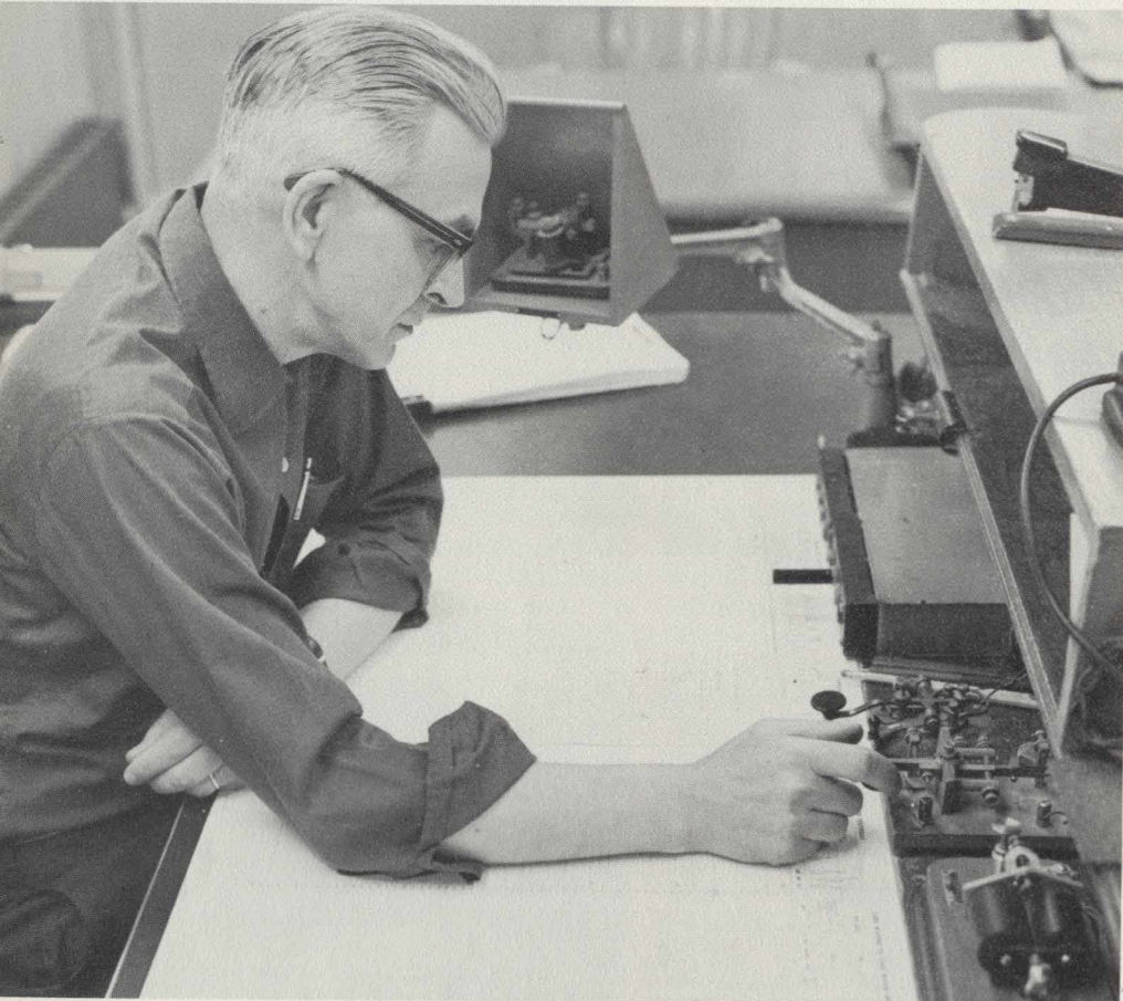
In August the telegraph will be a thing of the past on the Bangor and Aroostook. Now used only by car distributors like O. E. Ingerson, pictured at left, it will be replaced by a voice carrier communications system that will connect all stations and several offices throughout the system. The $63,000 system will save about 9% on the investment and will eliminate the need for station agents to know telegraphy.
