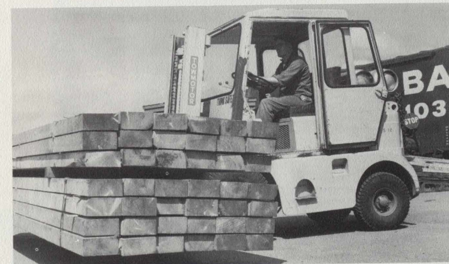
Above, worker using torch to cut scrap wears protective gloves, glasses and is careful not to stand under material that may fall on him. Below, fork lift operator keeps his load close to the ground to maintain stability.
