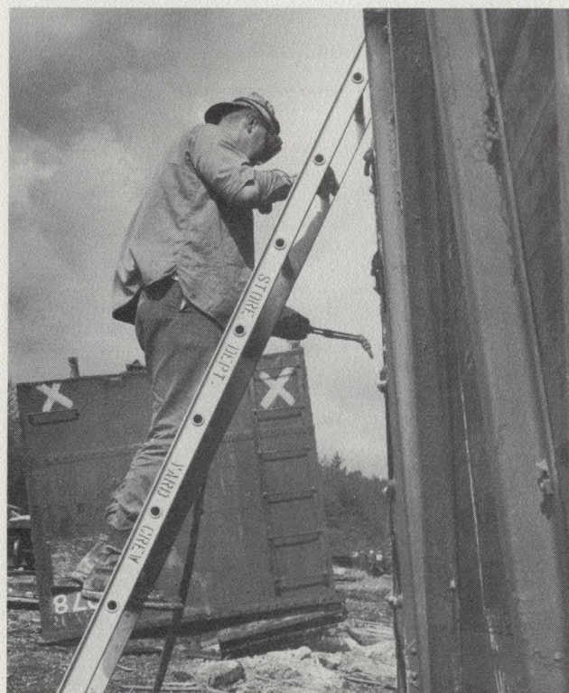
Workers pay special attention when attaching chains for the hook in handling scrap. Right, fork lift operator backs down ramp to maintain the stability of his machine. Below, worker on ladder uses proper hand holds and uses hard hat and protective glasses.
