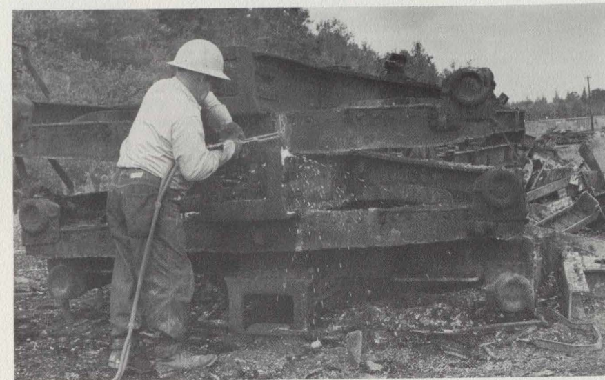
Above, worker using torch to cut scrap wears protective gloves, glasses and is careful not to stand under material that may fall on him. Below, fork lift operator keeps his load close to the ground to maintain stability.
