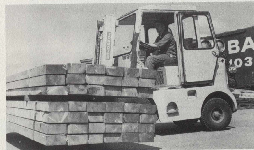
Above, worker using torch to cut scrap wears protective gloves, glasses and is careful not to stand under material that may fall on him. Below, fork lift operator keeps his load close to the ground to maintain stability.
