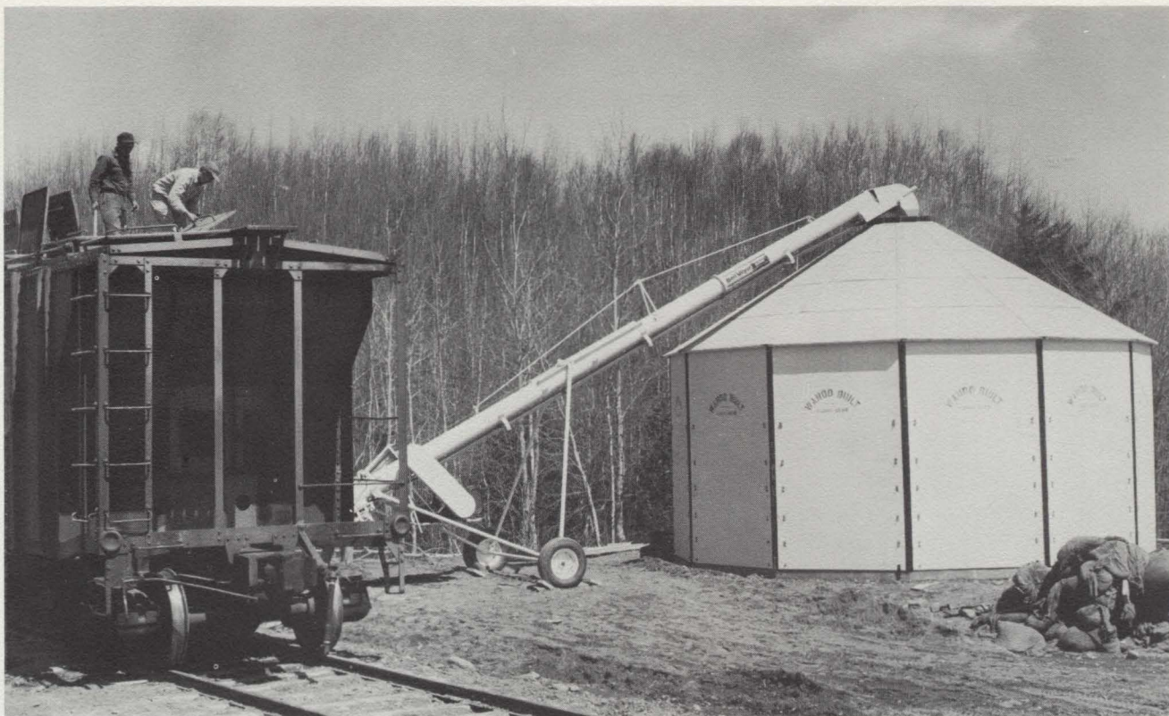
A mechanical device empties a heavily-laden fertilizer car into an igloo type storage silo at Houlton. The facility, located at the Donald Hagan potato house in Houlton, is one of two pilot projects of International Company for the merchandising of bulk fertilizer.
