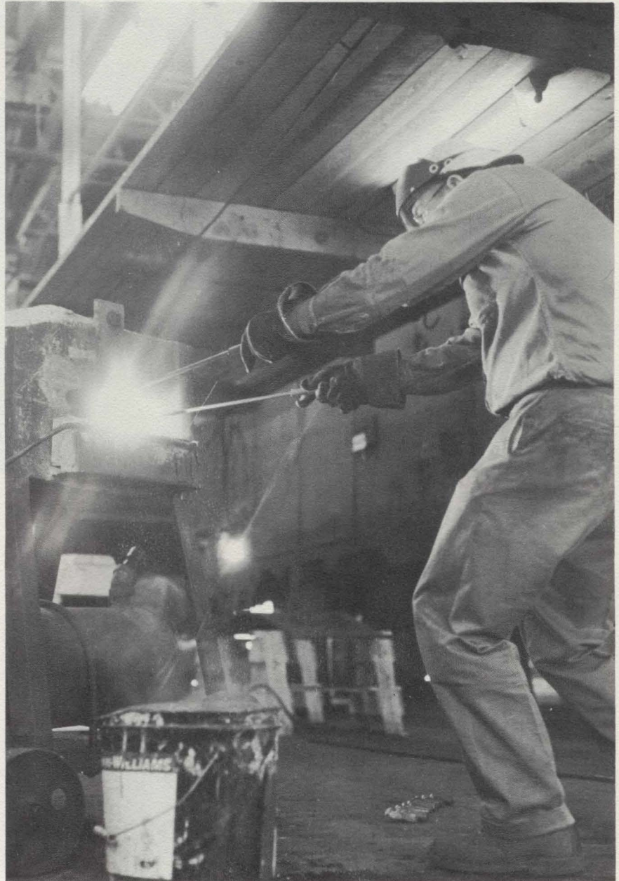
Perhaps the most nerve-wracking job, and certainly the hottest, in the assembly line reconditioning the cars is heating the rivets for the men working on the cars. The riveters depend on this man for a steady supply of glowing rivets that are tossed to them.
