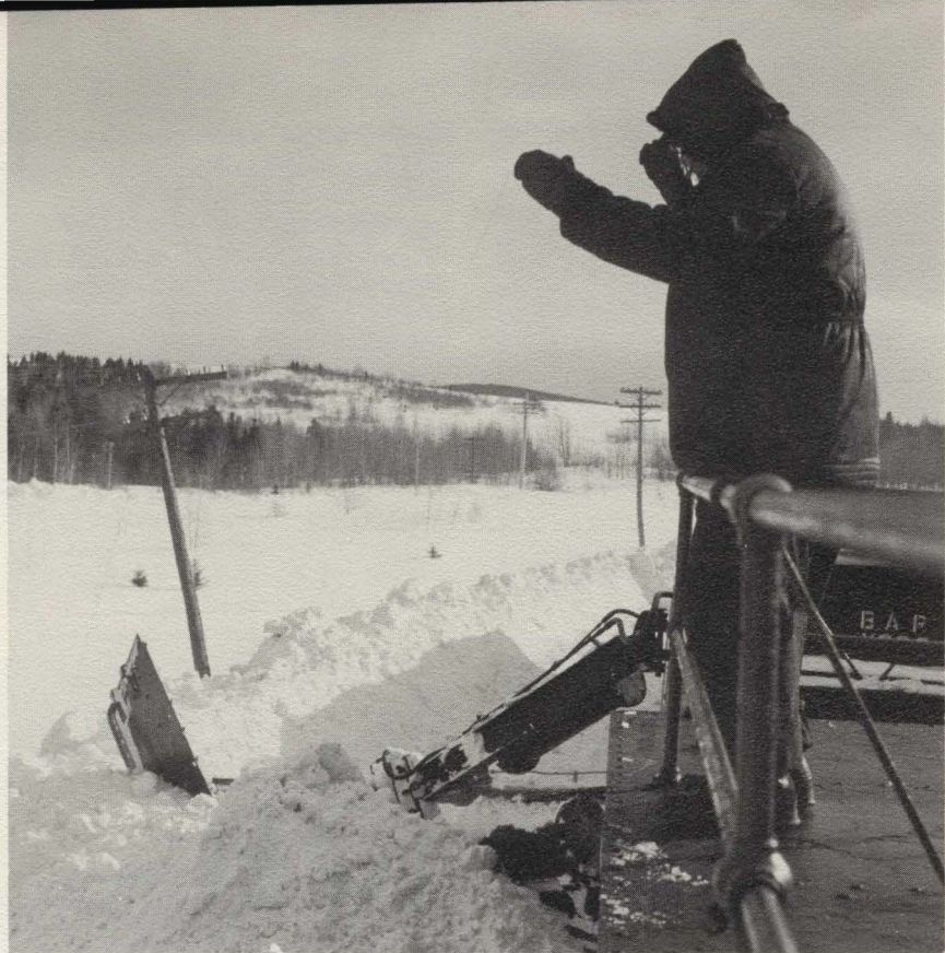
Spreader Foreman Joe Allen, bundled against bitter cold, signals spreader operator from his precarious perch. Below Pettibone snow blower bores its way through a bank at Oakfield yard.
