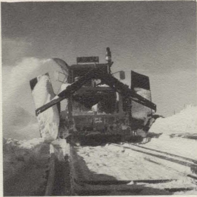
Kershaw ballast regulator
