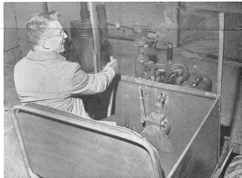
Steering controls of this snow cat are like those of a tank. Two separate braking systems lock each tread independently of the other, allowing the machine to turn literally on its own axis.
