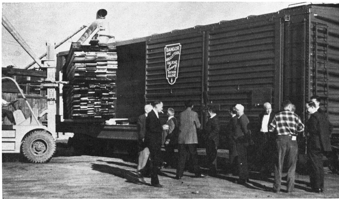
Top, new, experimental lumber car has extra-wide doors in each side to permit mechanical loading by fork lift. Center photograph from interior of car shows expanse of loading space when doors are opened. Bottom, the car is unloaded by fork lift at the R. A. Cleaves Planing Mill at South Portland as members of the New England Lumberman's association watch. The car was loaded at Pinkham's mill in Ashland. Unloading took only 45 minutes. (Bottom Photograph courtesy of the Portland Press Herald.)
