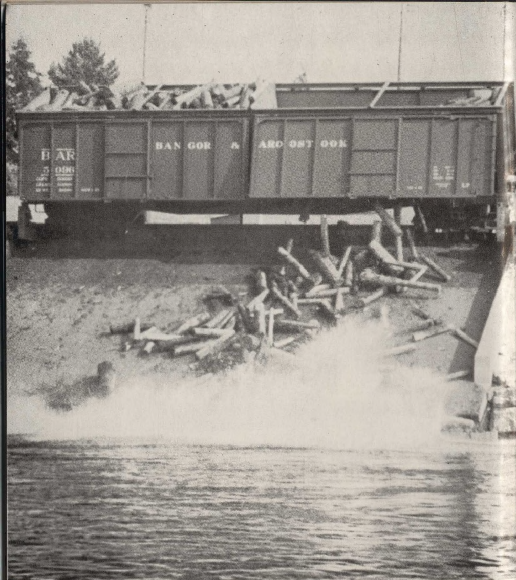
Pulp logs thunder down unloading chute at North Twin siding for the Great Northern mill. The Bangor and Aroostook side-dump cars shown above have saved countless man-hours of unloading time.
