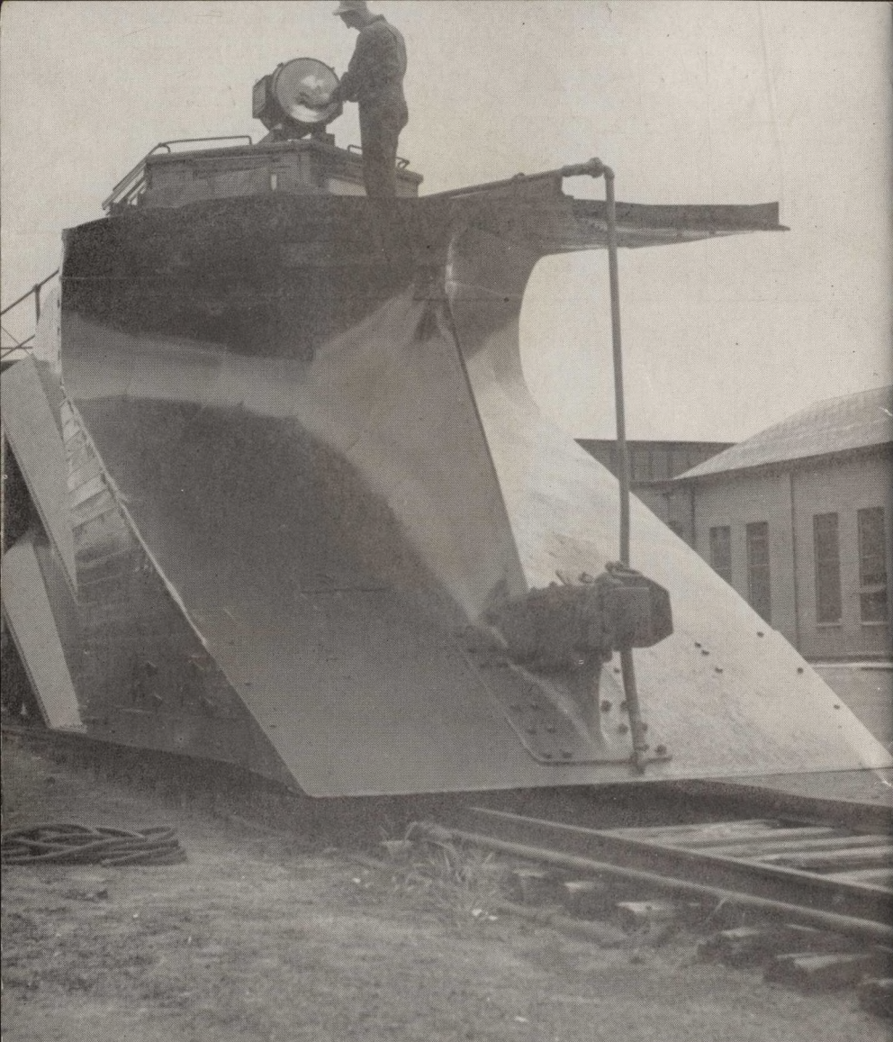
GETTING READY FOR WINTER —a newly reconditioned snow plow gets a lens replacement at Derby shops. Shining under a new coat of paint and rebuilt body the plow will be sent on the road to wait the first snow fall. A certain number of Bangor and Aroostook plows are reconditioned each year at Derby shops.
